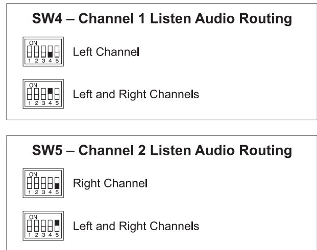
Figure 5. Channel 1 and channel 2 headphone audio routing mode configuration switches
